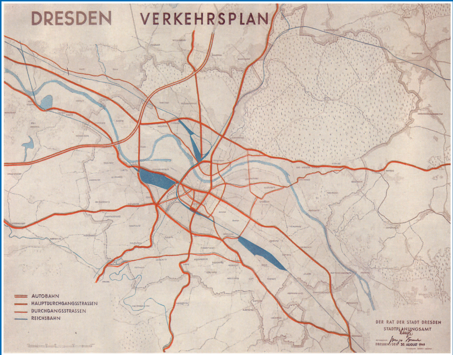
The Planned Main Road Network from the 1950s A tangent-formed system can be noted which is complemented by a link road leading over the river Elbe west of the city's 26 ring (former 26 tram line).
