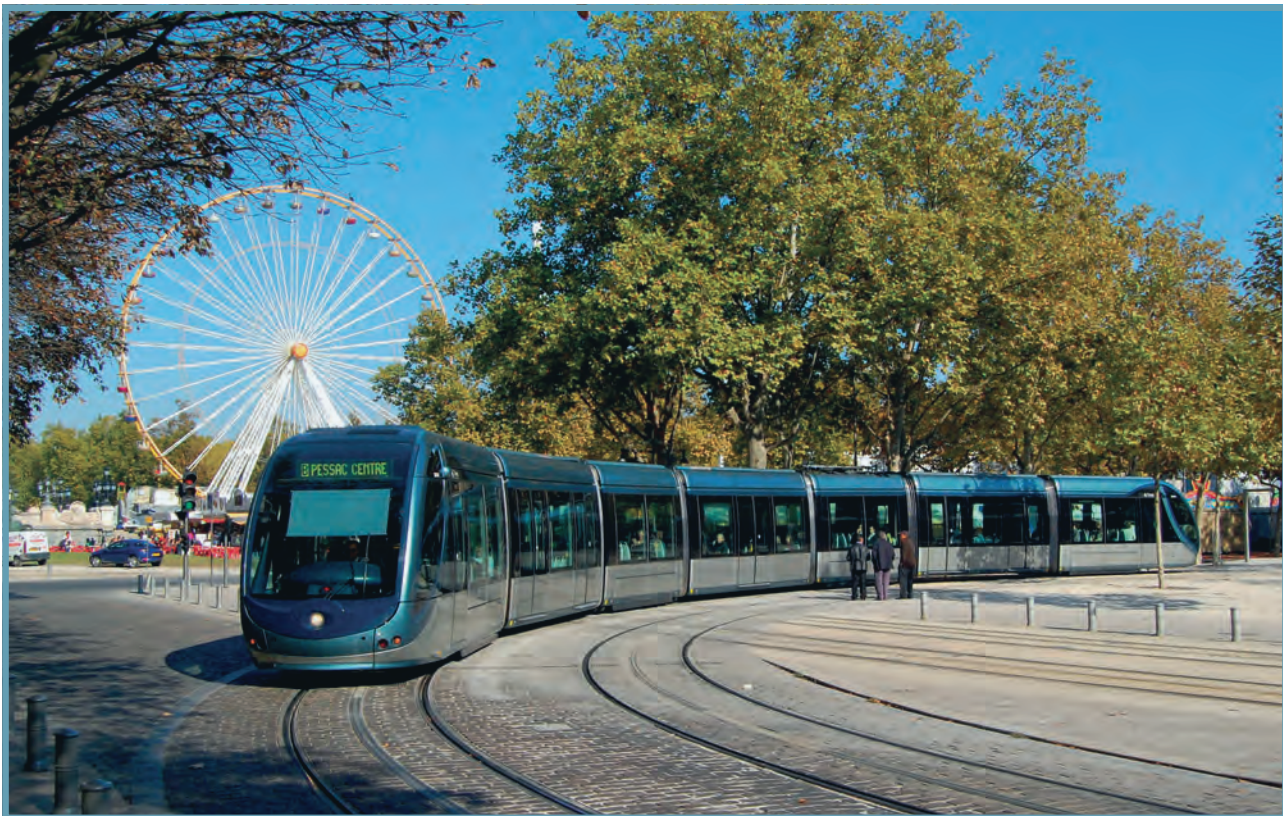
Figure 32: Alstom Citadis Tram in Bordeaux on Catenary-Free Section 41
