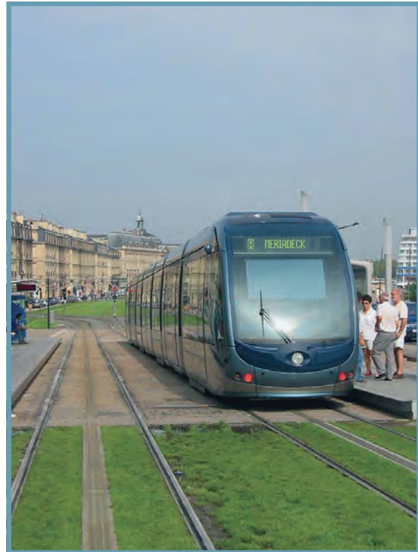
Figure 34: Citadis Tram powered by Third Conductor Rail 44
