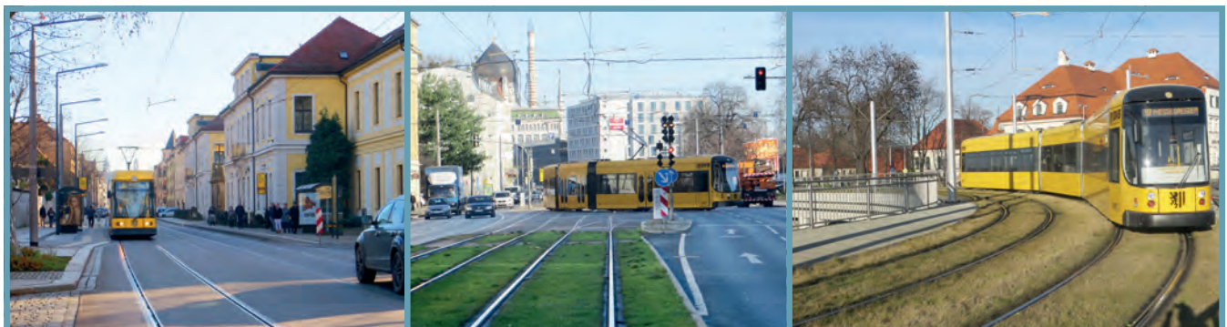
Figure 6: Flexibility of Different Types of Roadbeds (left: embedded, middle: separate, right: independent) 9
